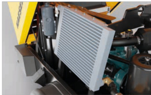
Compressed air aftercooler
