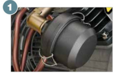
Air intake filter with silencer
