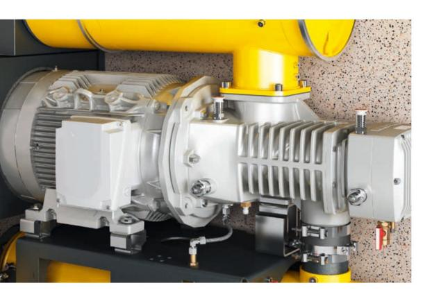
In CBS, DBS and EBS series rotary screw blowers, power is transferred from the motor to the blower airend via integrated gearing. This has proven to be the best solution for the prevailing speeds in this performance and size class when it comes to efficiency, reliability and durability. In the case of HBS series blowers, power is transferred directly, without losses, via a coupling. These design concepts are the result of extensive research at KAESER's Research and Development Centres.
