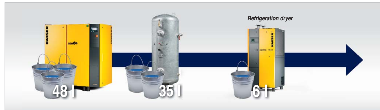
Fig. 1: Condensate occurs as a result of compressed air production, storage and treatment (figures based on 10 m 3 /min, 10 bar abs , 8 h, 60% H rel and 20 °C)
