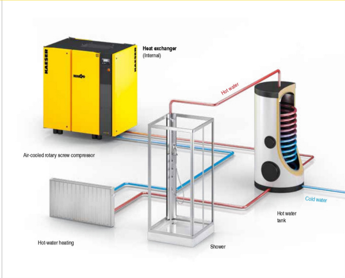
Image: Heat recovery process. Potable water applications only possible in conjunction with special, safety heat exchanger
